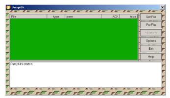
Click on Put File and Local file to be downloaded (Modbus\_TCP). 3. Enter password *G5* (case sensitive, must be upper case G) in **Remote file.** For **Remote host**, enter the IP address of the Micro PLC (for example: 10.10.0.2).
